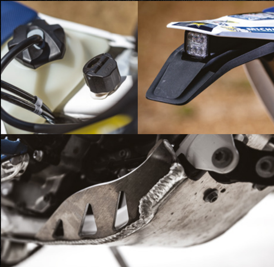
Top left: Fuel in the left oil in the right. Job Done. Top right: LED tail light. Above: Chunky alloy sump guard is available from the Husqvarna parts catalogue...
